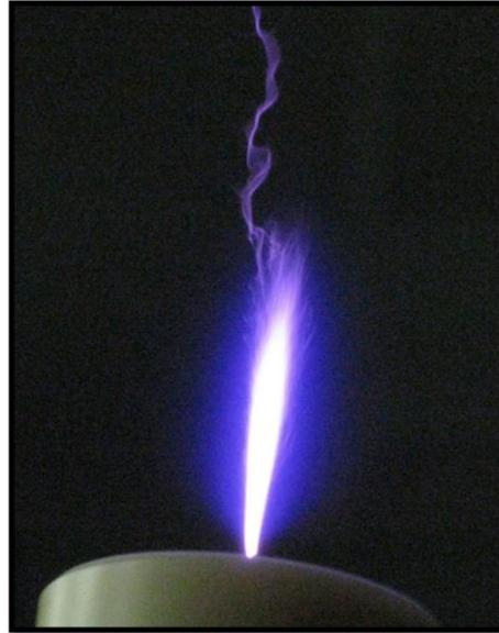
**Fig. 5.** 1.4÷1.6 MHz HF field is applied **to the cone**. All other details of the dynamic emitter are dielectric. Pressure in pre-chamber is 0.6 MPa.
