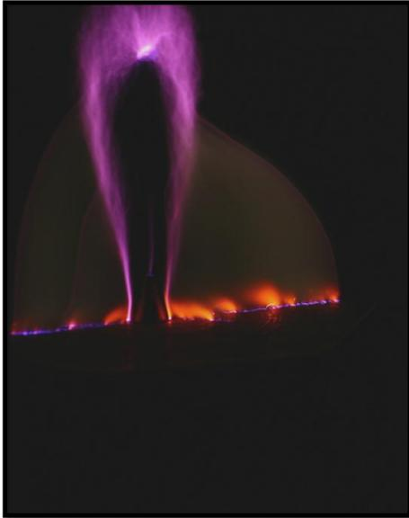
**Fig. 4.** An antenna is disposed at 10 cm **over the top** of the flow of grounded nozzle. 1.4÷1.6 MHz was supplied at antenna. Pressure in pre-chamber is 0.6 MPa.
