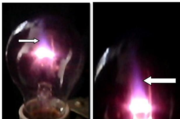
**Fig. 9-10.** Discharge between two wolfram spirals. Frequency 50 Hz, amplitude of current 10 mA, amplitude of voltage 1.5 kV. *Left* - general view with horizontal discharge, violet vertical column of the glow is directed against gravity. *Right* – zoomed view of the violet vertical column of the glow.
