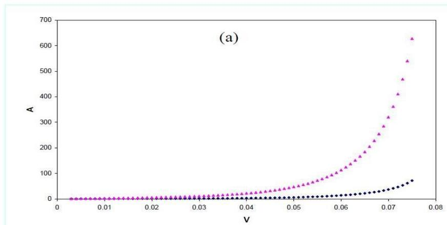
**Fig. 2-a.** Amplitude (A) versus velocity (v) for plasma (triangles) and scattered wave (squares) without relativistic effect included.
