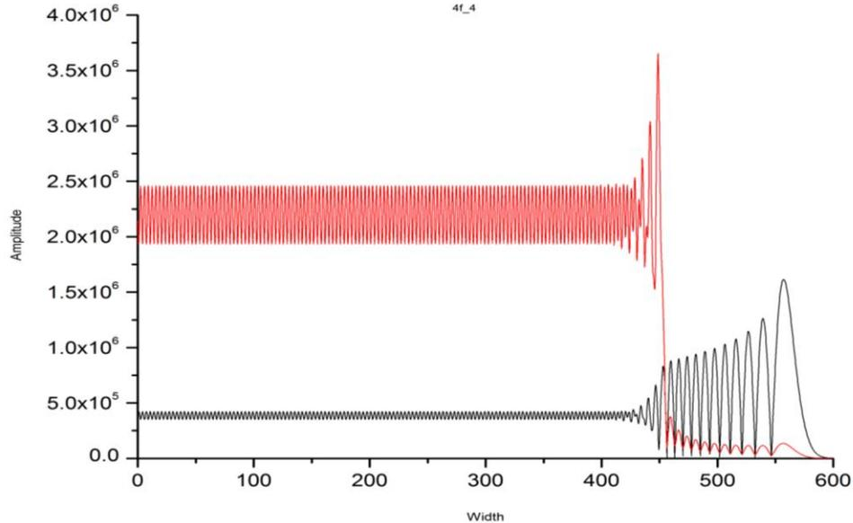
**Fig. 3.** Amplitude vs. width of the plasma slab for the amplified seed electromagnetic wave (black) and the coupled plasma wave (red). The preformed plasma channel extends to 2/3 of the plasma slab. The remaining third is inhomogeneous over dense plasma including the resonance and reflection points of both waves. The inhomogeneous density part extends from  $n_p / n_c = 0.15 - 0.44$ .
