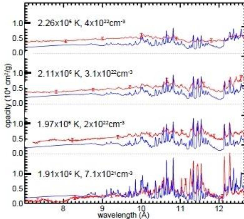
**Figure 6:** Measured iron opacity spectra (red) at four  $T_e/n_e$  values are compared with predicted values (blue) calculated using the SCRAM model which accounts for the instrument resolution. With higher temperature and density the measured opacity becomes more featureless while the background shows larger difference with the predictions<sup>[1]</sup>.
